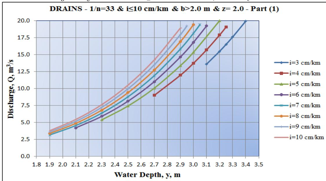
Fig-22. Design Chart for Drains of  $i \leq 10$  cm/km and  $b > 2.0$  m,  $z = 2.0$  and  $20 < Q < 80$  m<sup>3</sup>/s
