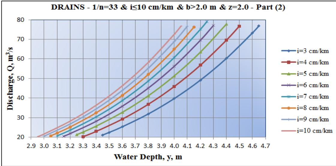
Fig-23. Design Chart for Drains of  $i \leq 10$  cm/km,  $b > 2.0$  m,  $z = 2.0$  and  $80 < Q < 200$  m<sup>3</sup>/s
