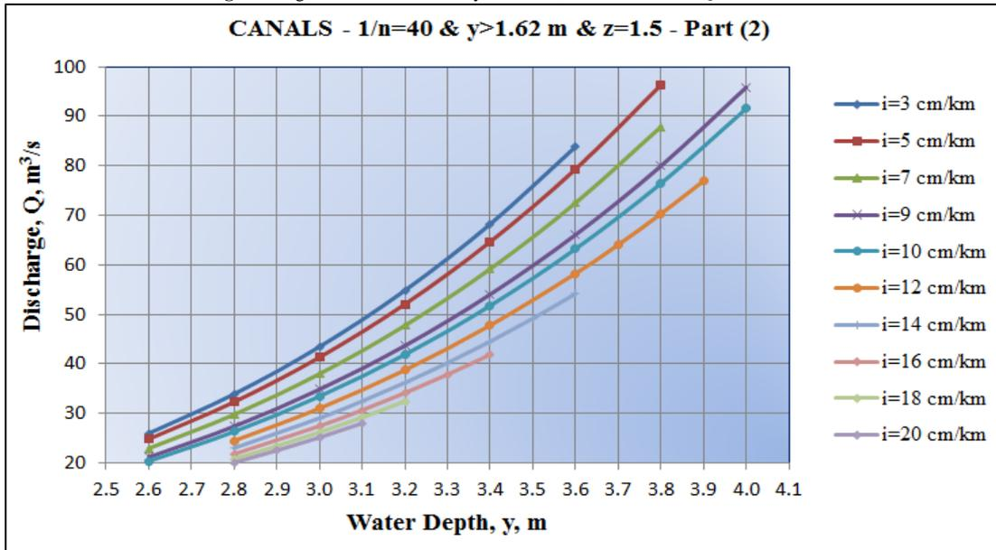
Fig-10. Design Chart for Canals of  $y > 1.62$  m,  $z = 1.5$  and  $100 < Q < 280$  m<sup>3</sup>/s
