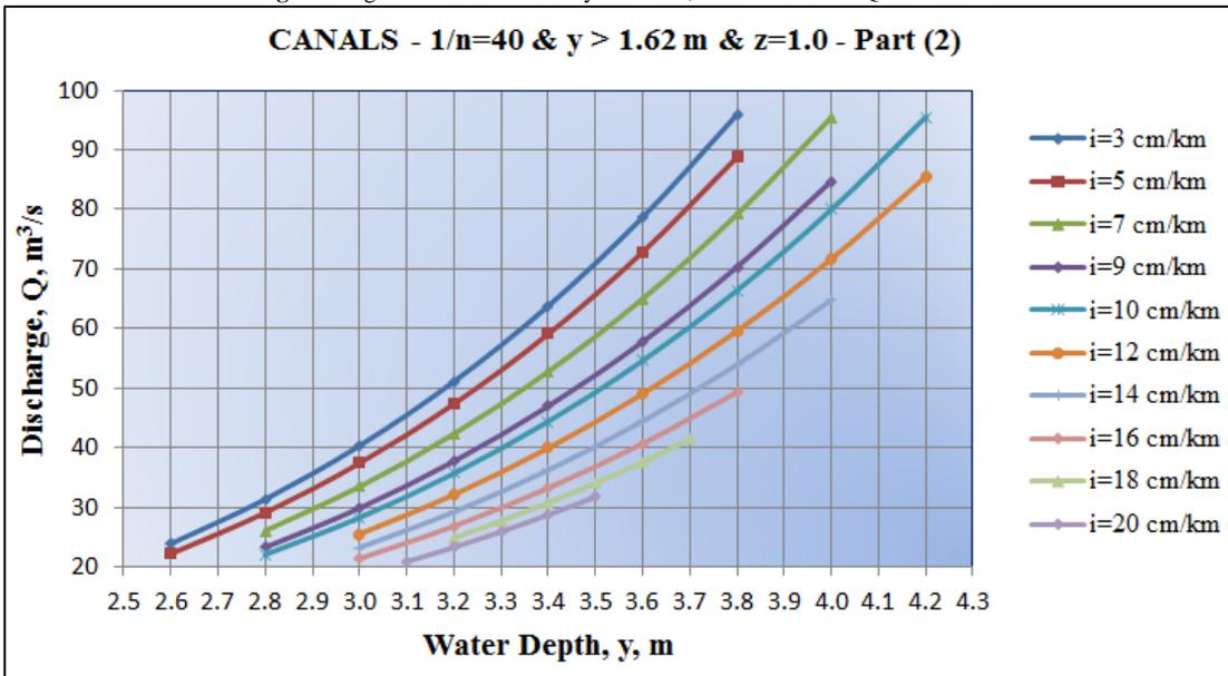
Fig-7. Design Chart for Canals of  $y > 1.62$  m,  $z = 1.0$  and  $100 < Q < 280$  m<sup>3</sup>/s
