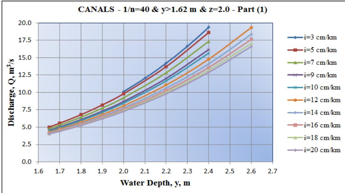
Fig-12. Design Chart for Canals of  $y > 1.62$  m,  $z = 2.0$  and  $20 < Q < 100$  m<sup>3</sup>/s
