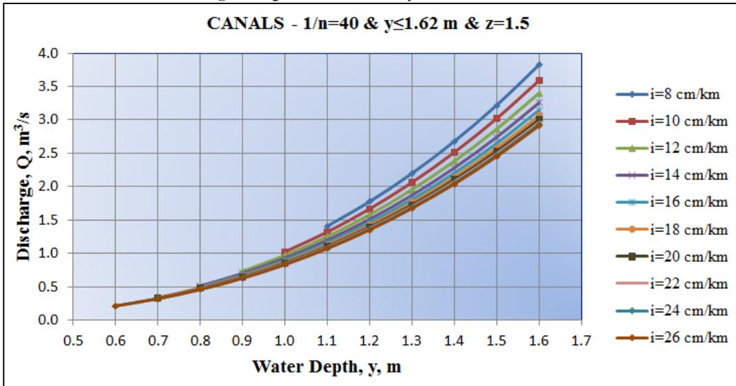
Fig-4. Design Chart for Canals of  $y \leq 1.62$  m and  $z = 2.0$
