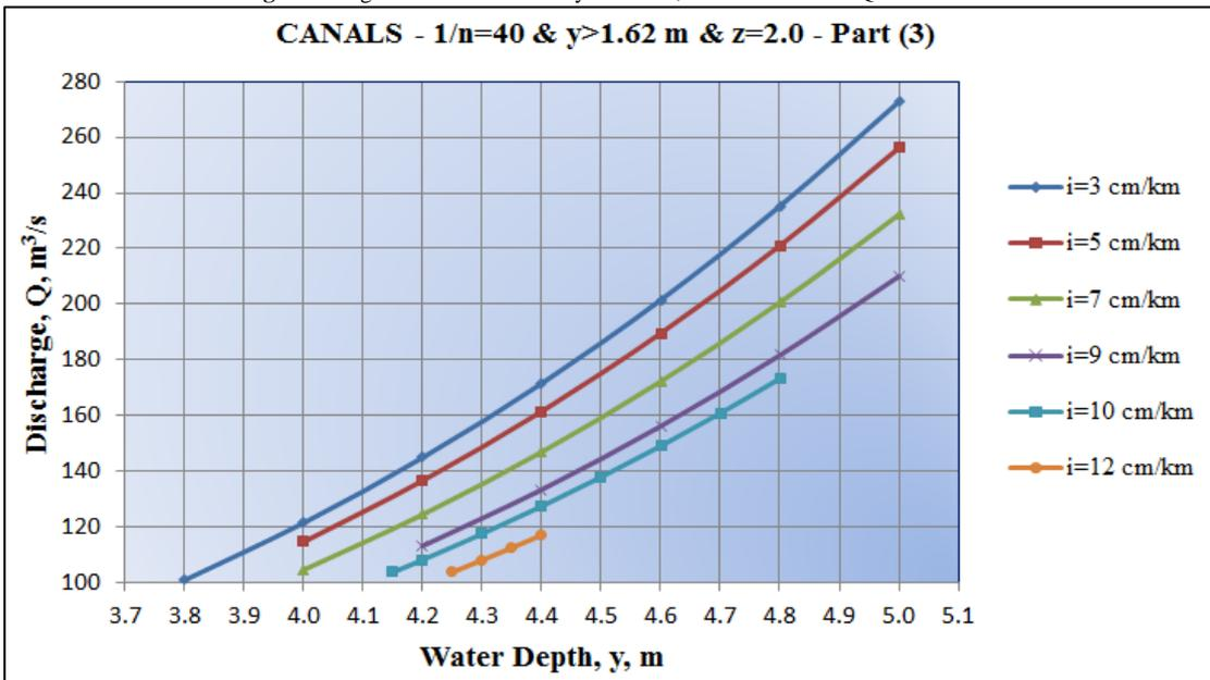
It could be seen from Fig. 5 through Fig. 13 concerning canals of  $y > 1.62$  m that the discharge increased as the longitudinal slope decreased at each specific water depth.
