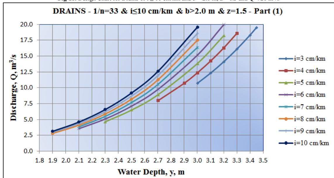
Fig-19. Design Chart for Drains of  $i \leq 10$  cm/km and  $b > 2.0$  m,  $z = 1.5$  and  $20 < Q < 80$  m<sup>3</sup>/s
