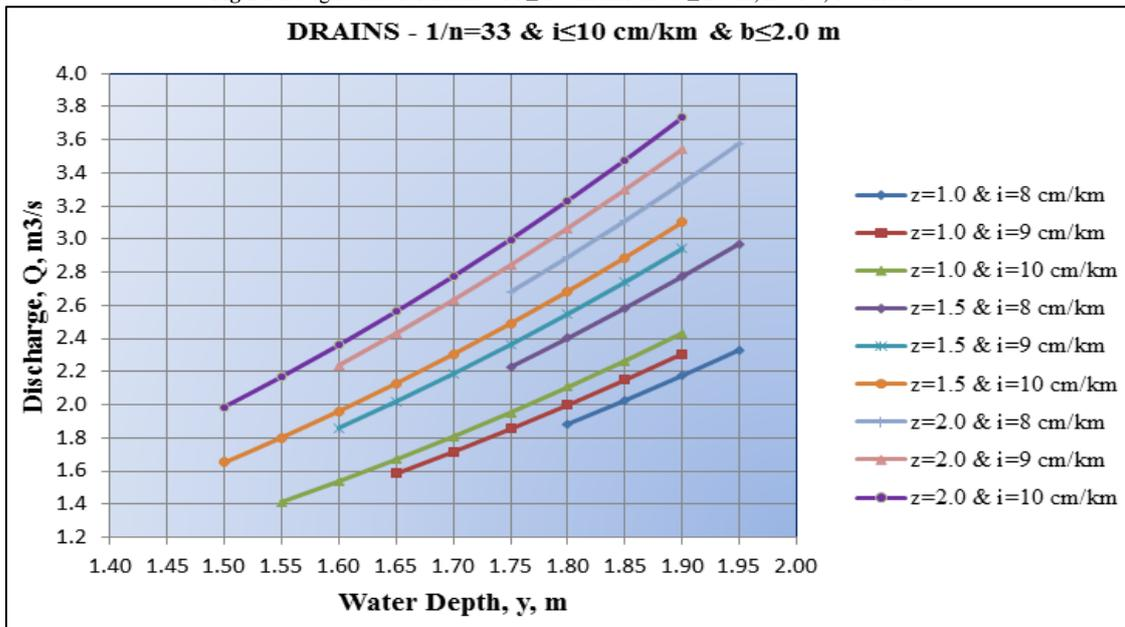
It could be seen from Fig. 14 concerning drains of  $i \leq 10$  cm/km and  $b \leq 2.0$  m that the discharge increased as the longitudinal slope increased at each specific water depth.
