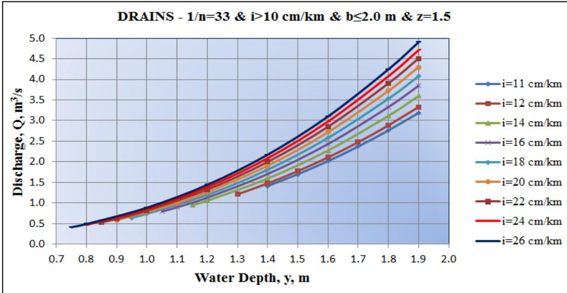
Fig-26. Design Chart for Drains of  $i > 10$  cm/km and  $b \leq 2.0$  m,  $z = 2.0$
