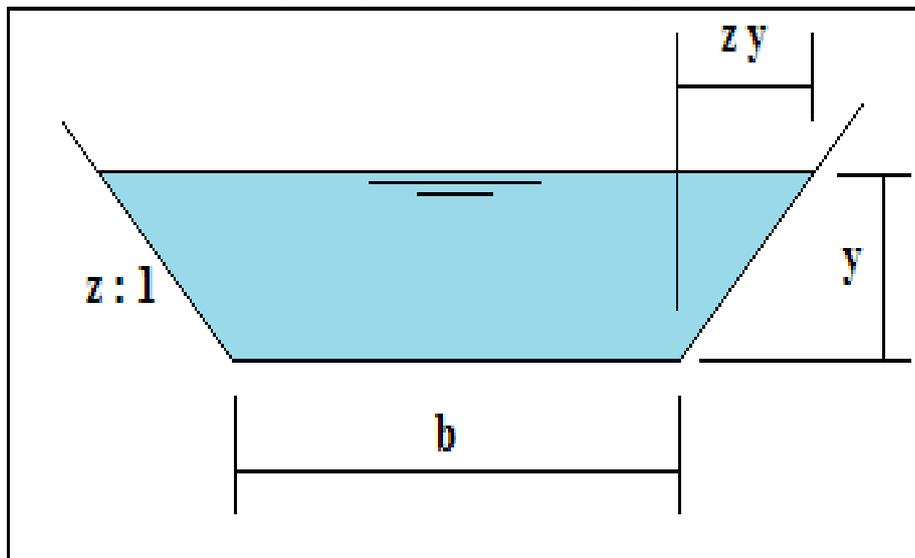
For average conditions, the value  $1/n$  is taken to be 40 for canals and 33 for drains, [22, 24]. The longitudinal slope is taken equal to the slope of the water surface ( $S = i$ ) to maintain a uniform flow of water through the channel. Three side slopes are studied representing different types of the soils. These side slopes are 1:1, 3:2 and 2:1, [22, 25].
