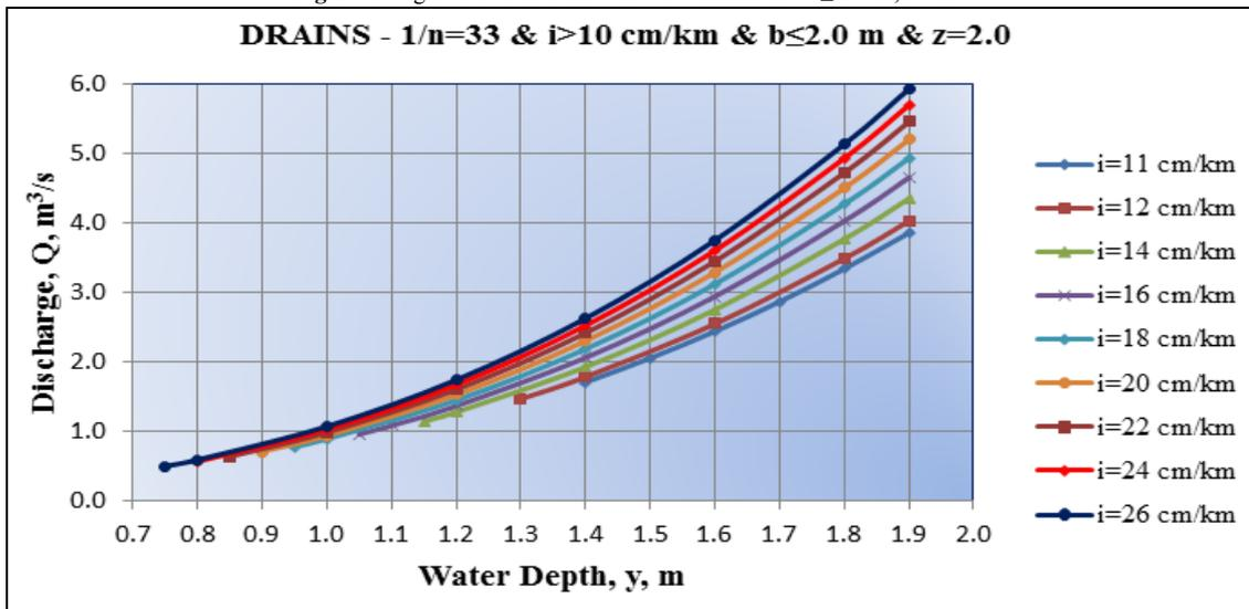
For drains of  $i > 10$  cm/km and expected  $b > 2.0$  m, Eq. 7 was applied with Manning equation for the three values of  $z$  and various values of  $i$  ( $S = i$ ). The obtained results were presented graphically forming design charts, as shown in Fig. 27 through Fig. 32.
