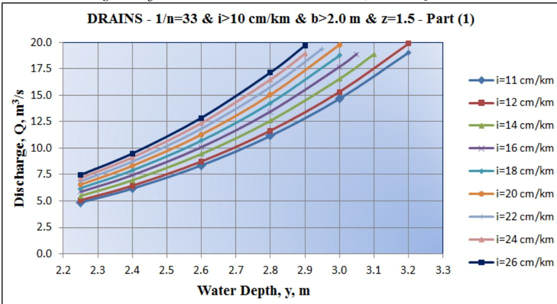
Fig-30. Design Chart for Drains of  $i > 10$  cm/km,  $b > 2.0$  m,  $z = 1.5$  and  $20 < Q < 160$  m<sup>3</sup>/s
