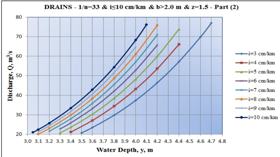
Fig-20. Design Chart for Drains of  $i \leq 10$  cm/km,  $b > 2.0$  m,  $z = 1.5$  and  $80 < Q < 200$  m<sup>3</sup>/s
