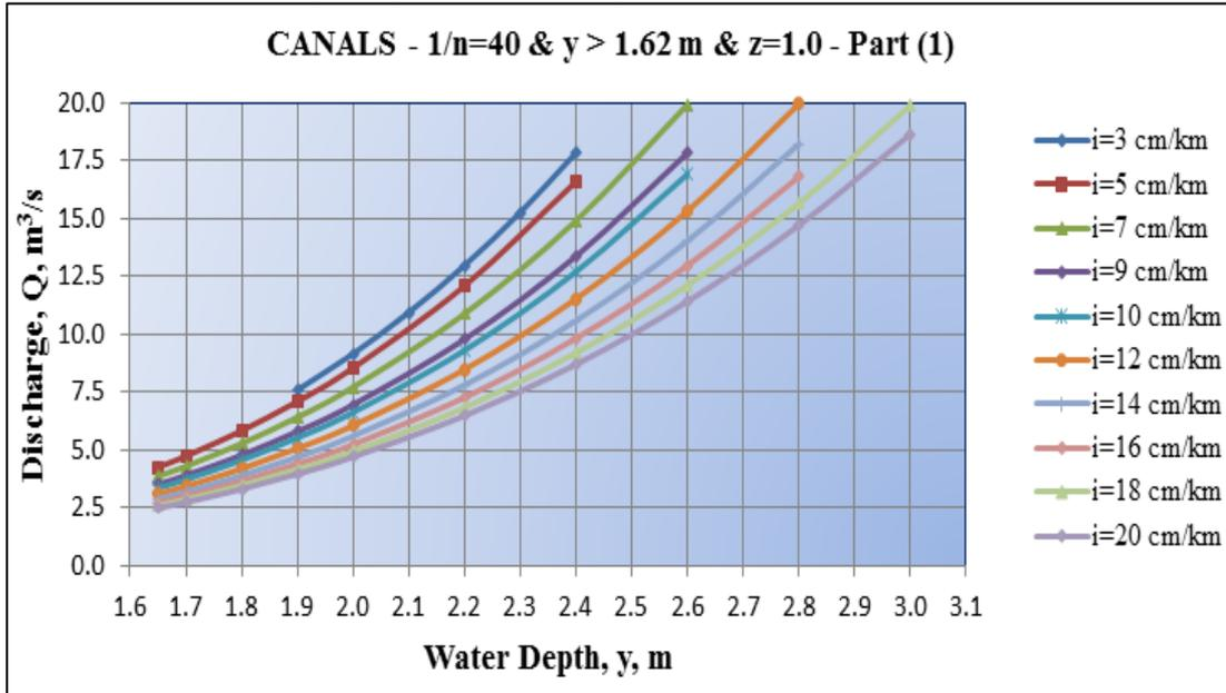
Fig-6. Design Chart for Canals of  $y > 1.62$  m,  $z = 1.0$  and  $20 < Q < 100$  m<sup>3</sup>/s
