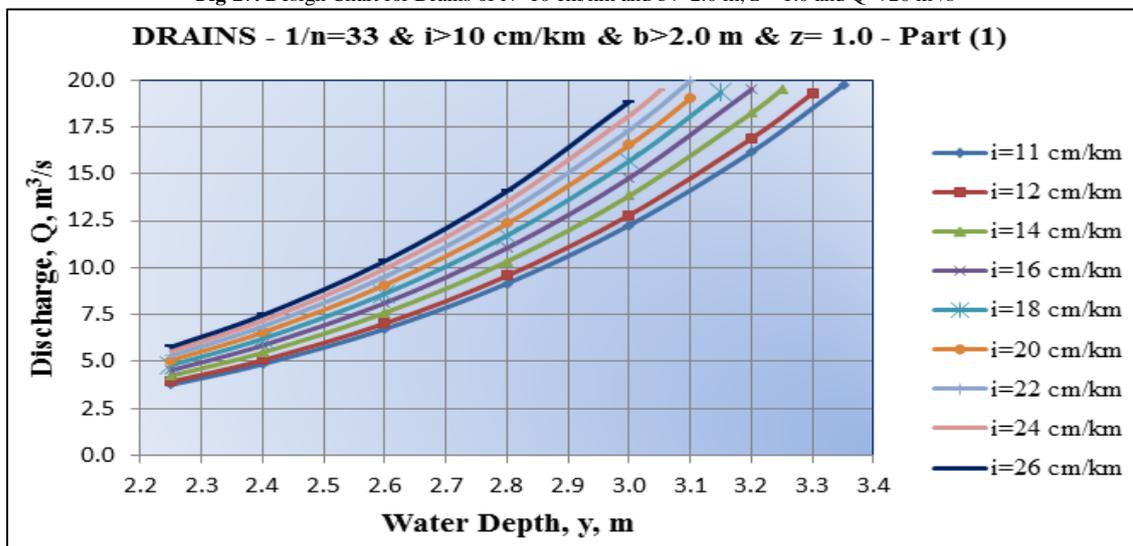
Fig-28. Design Chart for Drains of  $i > 10$  cm/km,  $b > 2.0$  m,  $z = 1.0$  and  $20 < Q < 140$  m<sup>3</sup>/s
