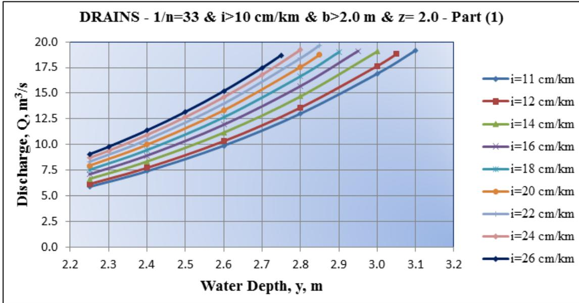
Fig.32. Design Chart for Drains of  $i > 10$  cm/km,  $b > 2.0$  m,  $z = 2.0$  and  $20 < Q < 160$  m<sup>3</sup>/s
