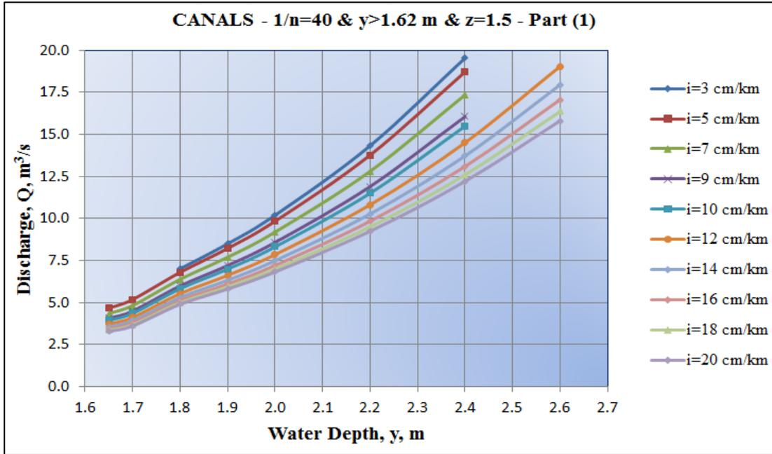
Fig-9. Design Chart for Canals of  $y > 1.62$  m,  $z = 1.5$  and  $20 < Q < 100$  m<sup>3</sup>/s
