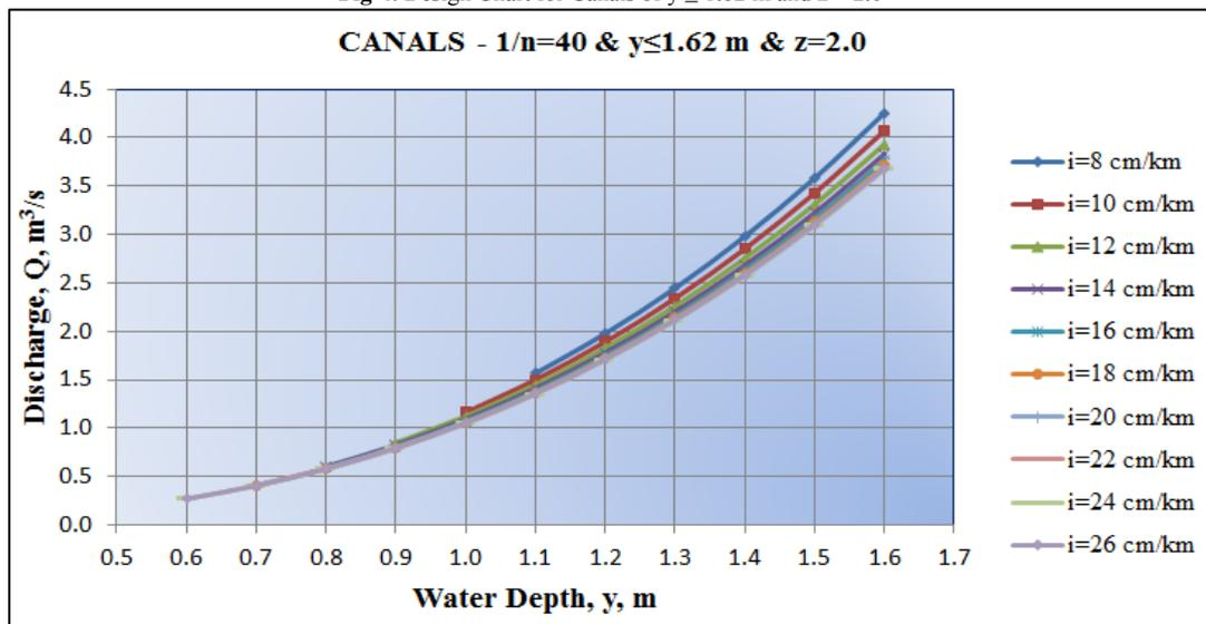
For canals of expected  $y \leq 1.62$  m, Eq. 2 was applied with Manning equation for various values of  $i$  ( $S = i$ ). The obtained results were presented graphically forming design charts, as shown in Fig. 5 through Fig. 13.
