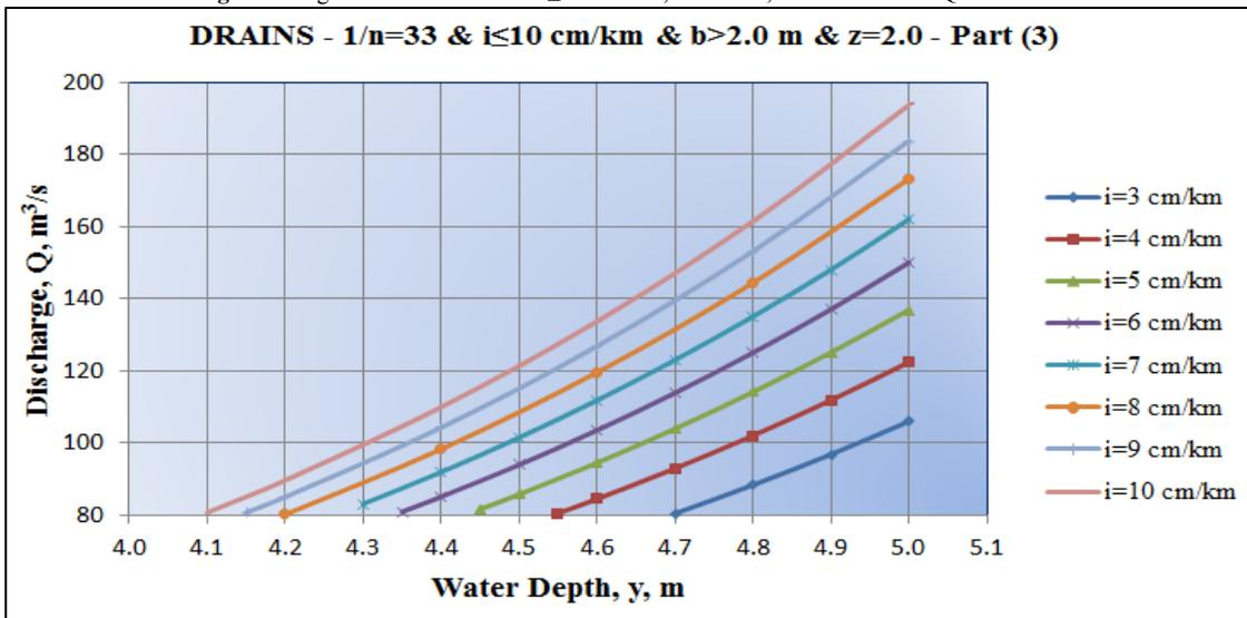
For drains of  $i > 10$  cm/km and expected  $b \leq 2.0$  m Eq. 6 was applied with Manning equation for the three values of  $z$  and various values of  $i$  ( $S = i$ ). The obtained results were presented graphically forming design charts, as shown in Fig. 24, Fig. 25 and Fig. 26.
