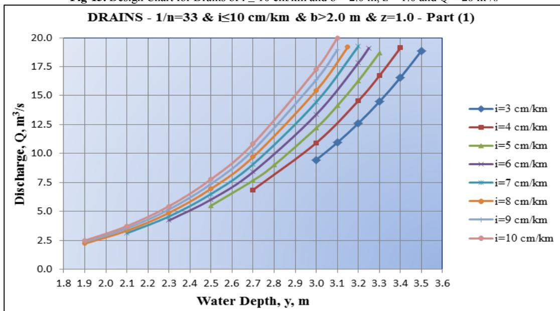
Fig-16. Design Chart for Drains of  $i \leq 10$  cm/km and  $b > 2.0$  m,  $z = 1.0$  and  $20 < Q < 80$  m<sup>3</sup>/s
