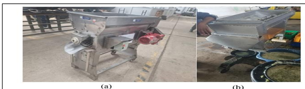
Figure-4. De stemmer machine (a) after fabrication and (b) during work
